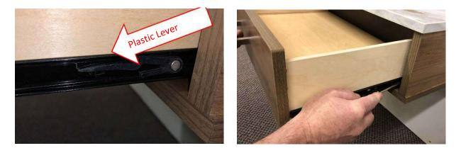
5. **RIGHT SIDE** - Place a flat tip screw driver into the gap between the cabinet side and drawer side – and move the lever downward. *When the lever moves - pull the right side of the drawer out slightly.*
