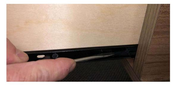
6. **LEFT SIDE** - Place a flat tip screw driver into the gap between the cabinet side and drawer side – and move the lever upward. *When the lever moves - pull the left side of the drawer out slightly.*
