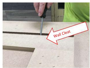
The Wall Cleats are held in place by small pins for shipping.
