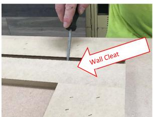
The Wall Cleats are held in place by small pins for shipping.
