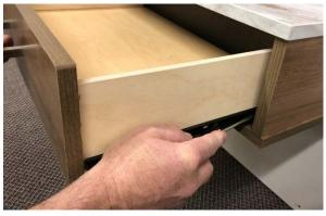
5. RIGHT SIDE - Place a flat tip screw driver into the gap between the cabinet side and drawer side — and move the lever downward. When the lever moves - pull the right side of the drawer out slightly.
